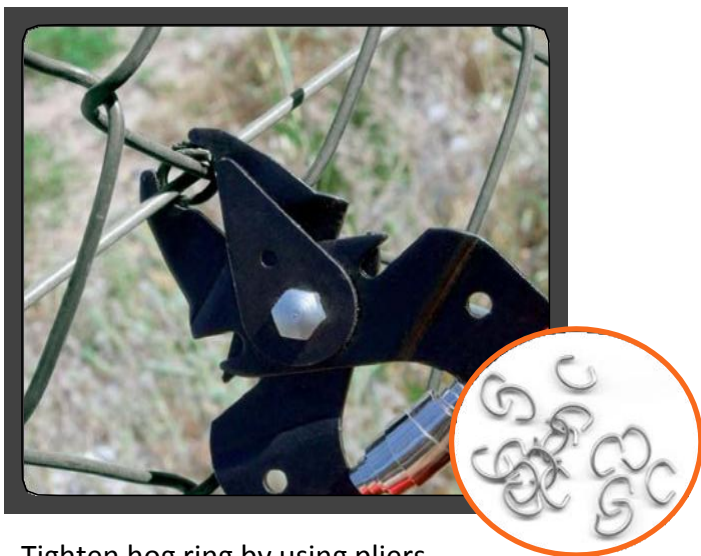
Tighten hog ring by using pliers
