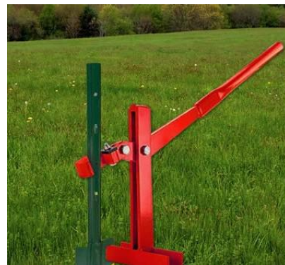
Post puller for U post uninstalling
